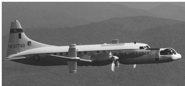
Fig. 2 General Dynamics total in-flight simulator (TIFS) research aircraft.
